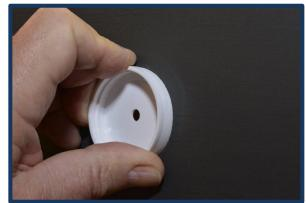
The fit is very tight and requires a board to completely press the cap in place. The board also assures that the cap becomes flush with the front surface of the fascia. Once the glue set, I tried to press the cap out of the fascia and it held tight. Mount your toggle switch in the cap and you're good to go!
