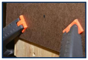
I use a 2 inch bit to bore the fascia. All fascias are made from ¼ inch thick Masonite. Any areas that require a severe bend are two thicknesses of 1/8 inch Masonite bonded together.
